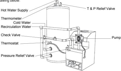
If this water heater is installed in a closed water supply system, such as one having a back-flow preventer in the cold water supply line, means shall be provided to control thermal expansion. Contact the water supplier or local plumbing inspector on how to control this situation.
